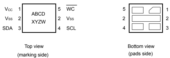
Figure 3. UFDFPN5 (DFN5) package connections
