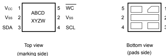
Figure 3. UDFPN5 (DFN5) package connections
