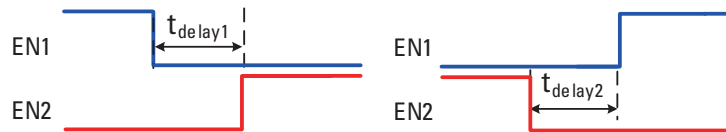
Figure 2. EN1 and EN2 Timing Control Diagram
